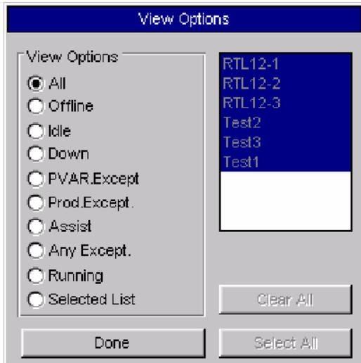
The *View* button opens the **View Options** window. This window filters the list of machines that appear on a **Monitor** window. The filtering is done by machine state or a selected machine list. Click on one of the circles to the left of the desired machine state. The **Monitor** window immediately changes its list of machines to those that are currently in the selected machine state.
